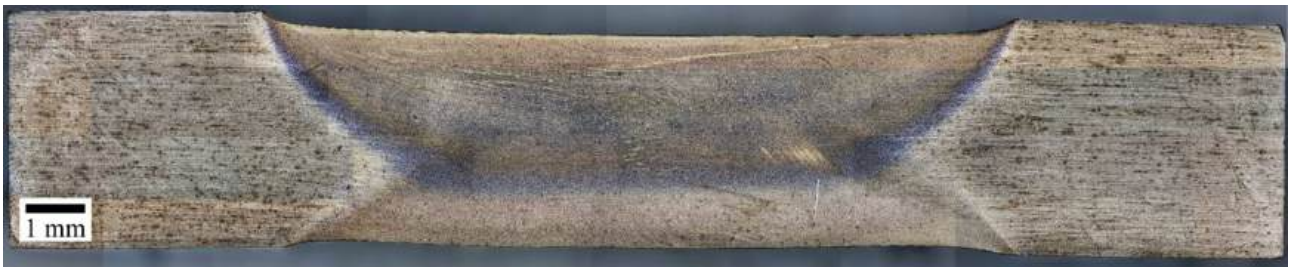
Fig. 2. Cross section of FSW joint of 0.15C steel.
