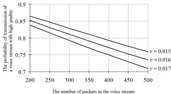
**Fig. 3.** Dependence of a high-quality stream transmission probability on the number of transmitted packets in a voice stream ( $v$  is the probability of packet loss during transmission)
