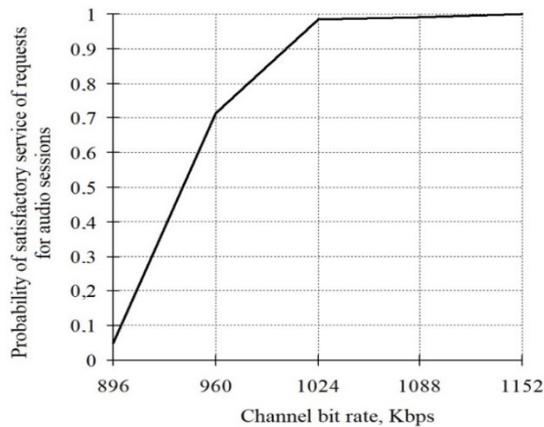
**Fig. 2.** Dependence of request satisfactory service probability for audio communication sessions on the channel bit rate
