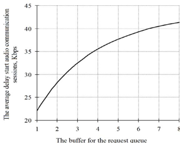
**Fig. 1.** Dependence of the average delay of audio communication session start on the buffer size for a request queue
