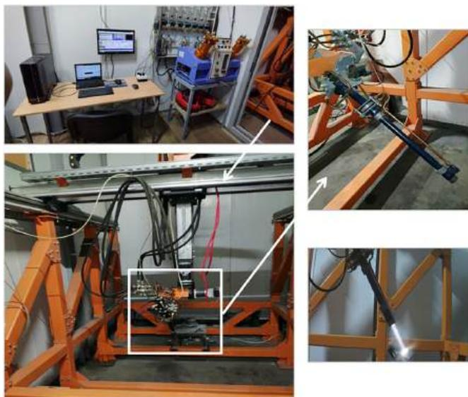
Fig. 2. A new robotic complex for detonation spraying of coatings (IntelMashin LLC, Russia) equipped with a multi-chamber detonation accelerator (MCDS).
