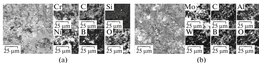
**Fig. 3.** Surface elemental distribution of composite metal–ceramic targets according to energy-dispersive X-ray spectroscopy: (a) Ni–Cr–B<sub>4</sub>C; (b) Mo–Al–W–B<sub>4</sub>C.
