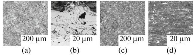
**Fig. 2.** Surface (a, c) and cross section (b, d) of composite metal–ceramic target: (a, b) Ni–Cr–B<sub>4</sub>C; (c, d) Mo–Al–W–B<sub>4</sub>C.
