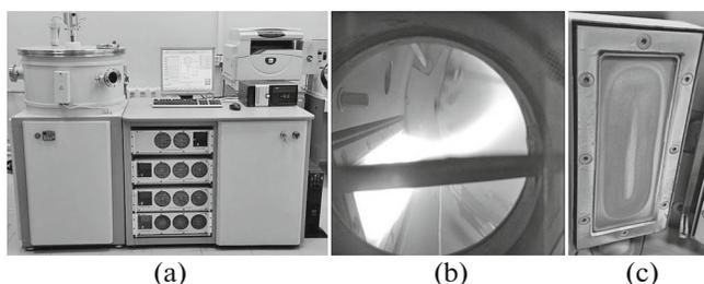
**Fig. 4.** External appearance of UniCoat 200 vacuum unit (a); magnetron sputtering with composite metal–ceramic target (b); and surface of target after sputtering (c).
