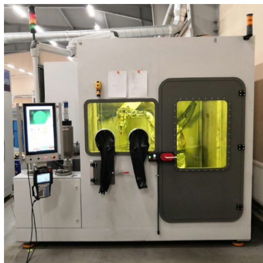
Figure 2. ILIST-M robotic complex for laser direct energy deposition.
