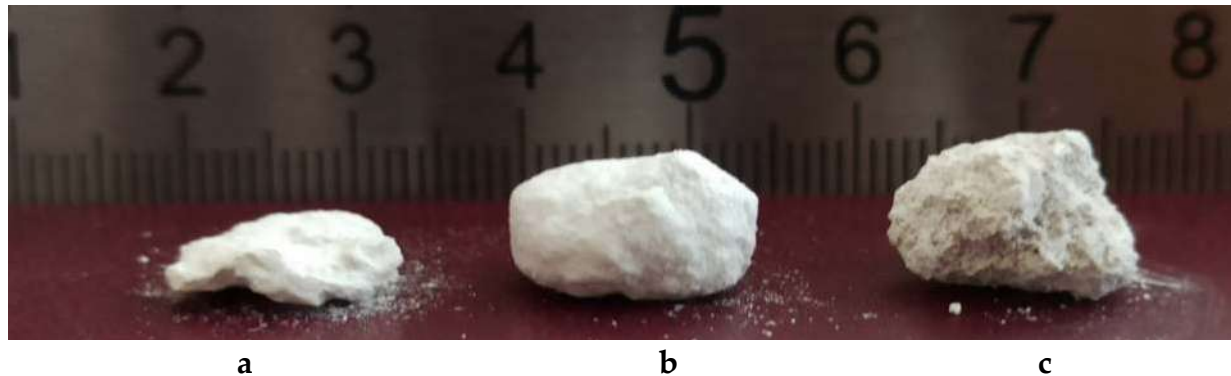
Figure 5. PG conglomerates with a size greater than 10 mm. (a)— PG_{Bel} ; (b)— PG_{Bal} ; (c)— PG_{Kin} .
