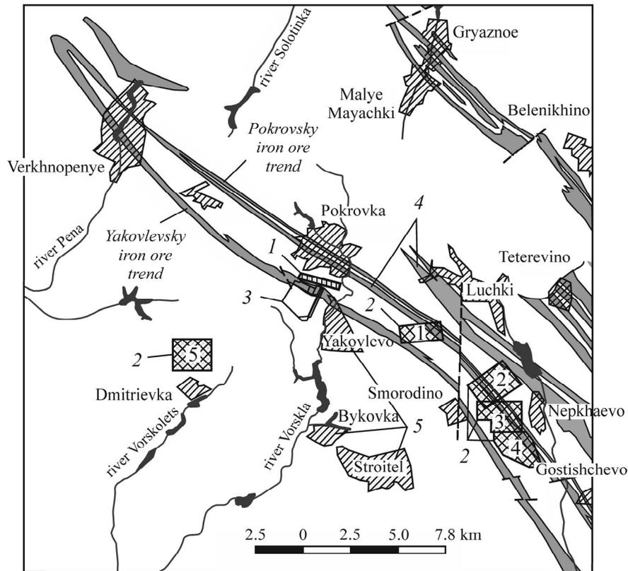
**Fig. 1.** Drain water injection sites under study: 1—drainage area; 2—drain water injection sites; 3—stopes; 4—ore trends; 5—inhabited localities.
