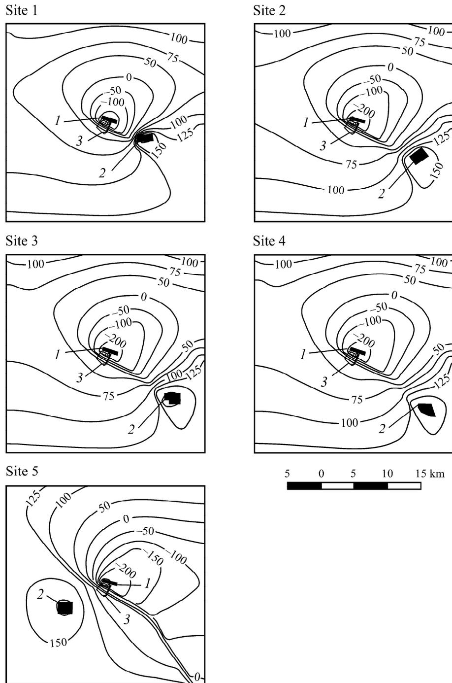
**Fig. 2.** Predictive distribution of level of water-bearing bottom coal layer at joint operation of drainage system and drain water injection sites (m abs.): 1—pumping site; 2—injection site; 3—stopes.
