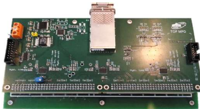
Fig. 3. NINO based 24-channel amplifier-discriminator with the Molex CXP connector.
