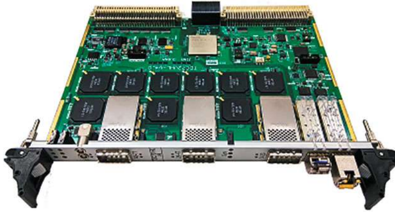
Fig. 4. 72-channel time-to-digital converter TDC72VHL v4 with CXP input connector.
