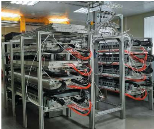
Fig. 5. Setup for testing the modules of the TOF system.
