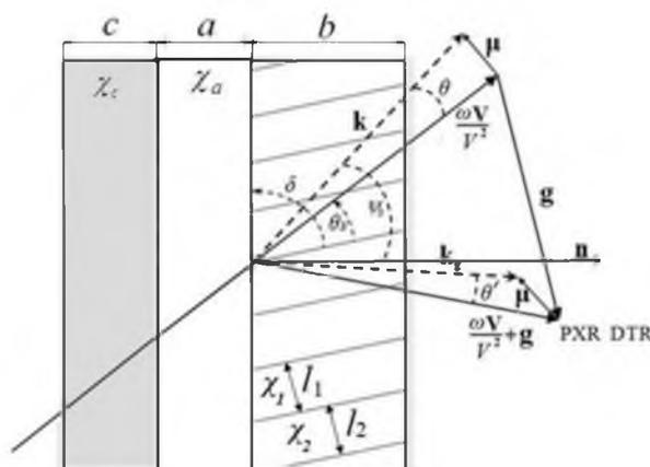
Fig.1. Geometry of the radiation process and the system of the using parameters notations,  $\theta$  and  $\theta'$  are the radiation angles,  $\theta_B$  is Bragg angle,  $\mathbf{k}$  and  $\mathbf{k}_g$  are wave vectors of incident and diffracted photons.
