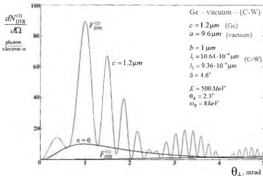
Fig.3. The angular density of DTR by a relativistic electron from three-layered structure and the same in case of absence ( $c=0$ ) of the amorphous layer. The angular density of PXR under such energy of electrons is considerably lower and independent on thickness of amorphous layer.
