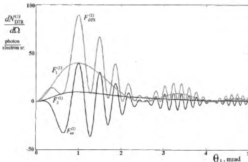
Fig. 4 The contribution of TR from the amorphous layer  $F_1^{(1)}$ , from the entrance boundary of the multilayered medium  $F_2^{(1)}$  and their interference term  $F_{int}^{(1)}$  into the angular density of DTR.
