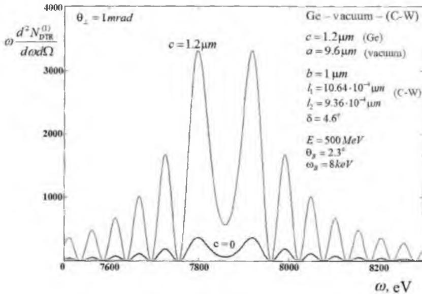
Fig.2 Spectral-angular density of DTR in the three-layer structure ( $c = 1.2 \mu\text{m}$ ) and in the case of absence of amorphous layer ( $c=0$ ).
