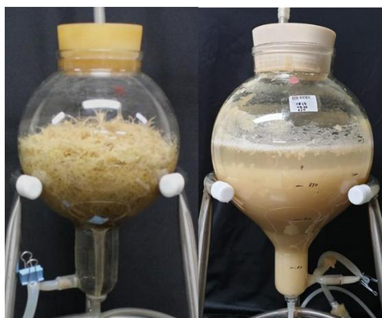
*Fig. 1. Bioreactor system for adventitious root (left) and cell suspension (right) cultured in medicinal plants.*
