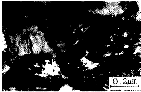
Fig. 5. Microstructure of Ti-6%Al-3.2%Mo alloy after deformation at \dot{\epsilon} = 5 \cdot 10^{-4} \text{s}^{-1} and T = 700^\circ\text{C} up to \epsilon = 5\% .
