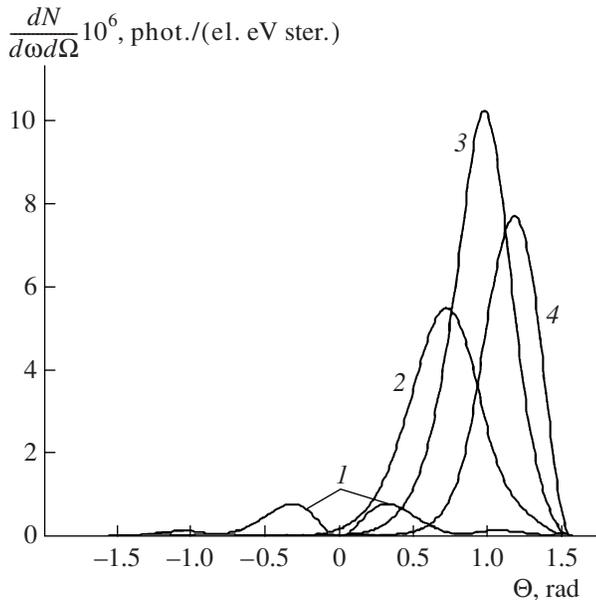
**Fig. 1.** Increase in the angular density of TR at  $\omega = 50$  eV for electrons with an energy of  $\varepsilon = 0.5$  MeV incident on the medium–vacuum interface at various angles  $\varphi = \pi/2$  (1), 0.7 (2), 0.45 (3), and (4) 0.2.
