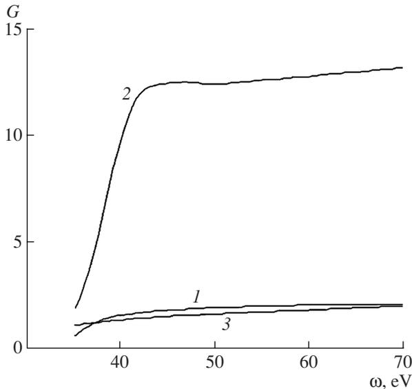
**Fig. 2.** Suppression of the effect of increase in the angular density of TR as manifested by the ratio  $G$  of the TR intensities at the maxima of angular distributions for the grazing (optimum  $\varphi$ ) and normal incidence angles at an electron energy  $\varepsilon$  of (1) 0.05, (2) 0.5, and (3) 5 MeV.
