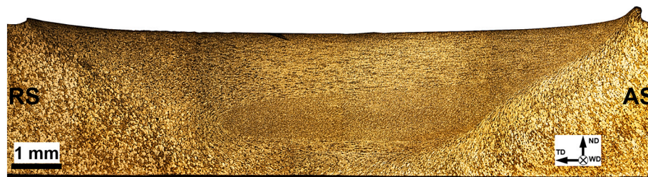
Fig. 4. Typical optical image of the weld cross-section. RS and AS denote the retreating side and advancing side, respectively. Note: The image of the 1100–125 weld is shown.
