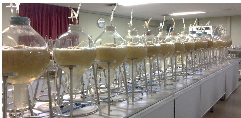
Fig. 1. Adventitious root culture in bioreactor system for the production of pharmacology active
