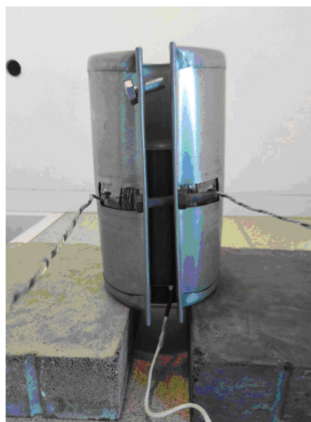
Fig. 1. Photograph of a mold design with a heating device.
