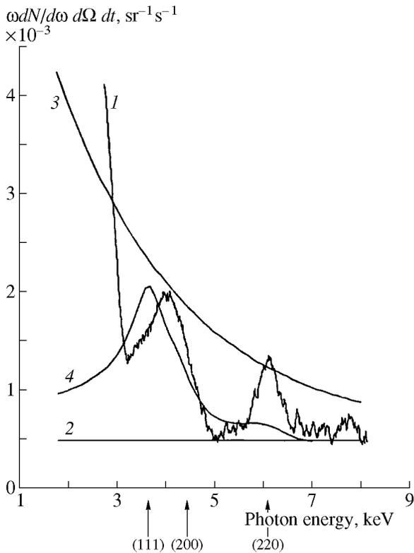
**Fig. 2.** Spectral distribution of polarization-bremsstrahlung intensity: (1) experimental data upon external-background subtraction; (2) conventional-background intensity; and (3, 4) calculated intensities of polarization bremsstrahlung and conventional background in an amorphous and in a polycrystalline aluminum target, respectively.
