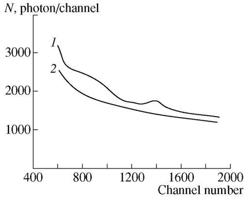
**Fig. 1.** Experimental spectrum of x-ray radiation generated by 2.4-MeV electrons in an aluminum target 2  $\mu\text{m}$  thick (spectral section above the K-line of aluminum): (1) main signal and (2) external background.
