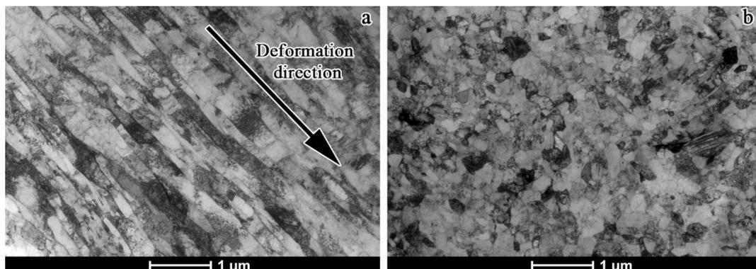
Figure 1. TEM bright-field images of a structure of the program steel in *a* longitudinal and *b* transversal section.
