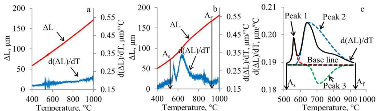
Figure 2. a dilatometric curve ( $\Delta L$ ) and  $d(\Delta L)/dT$ -curve of the pure nickel sample and b the program steel; c the sketch explaining  $d(\Delta L)/dT$ -curve for the program steel.
