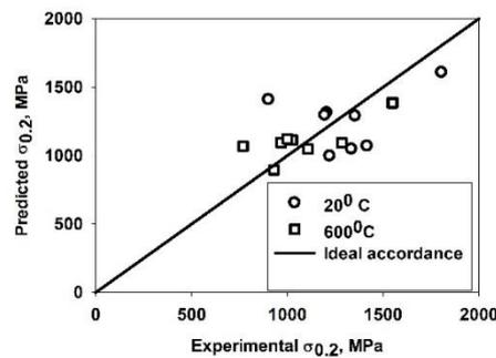
**Figure 2.** Experimental and predicted yield strengths at 20 and 600 °C.
