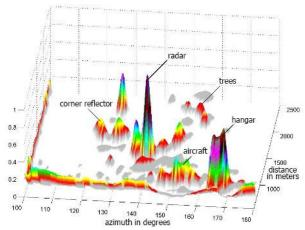
Fig. 4: The value of the normalized Euclidean norm of expectation vector difference for the analysis plots and bordering fragments.
