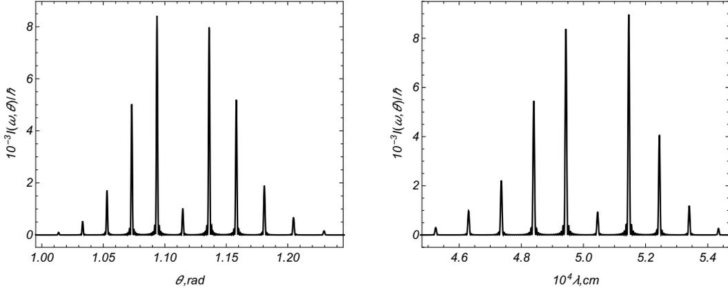
**Figure 1.** The angular (left panel) and wavelength (right panel) dependence for the intensity of the transition radiation on a plate made of fused quartz excited by two acoustic waves with uncorrelated phases.
