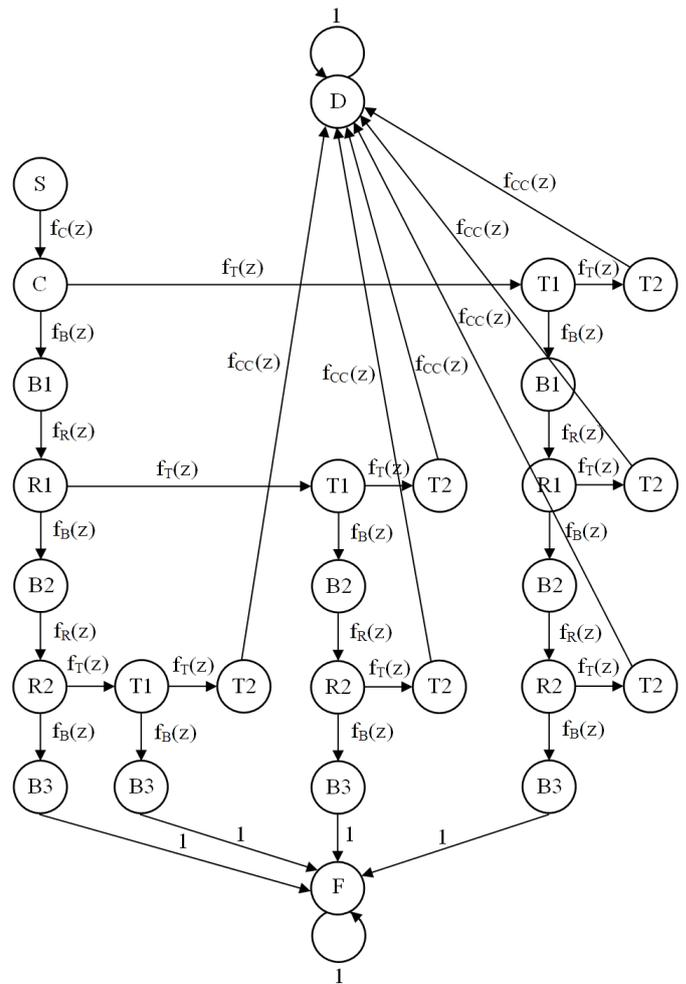
Fig. 1. Probability-time graph, modeling data transfer to MANET at  $m=2$  and  $n=2$ .
