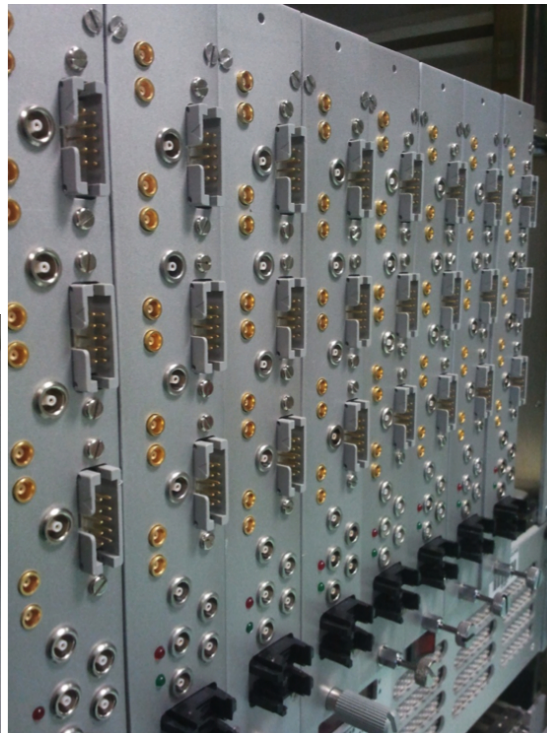
Figure 11: Left: A complete module with the inputs and connections to the feedthroughs; Right; the front panels with the analog and LVDS outputs
