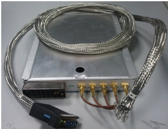
Figure 11: Left: A complete module with the inputs and connections to the feedthroughs; Right; the front panels with the analog and LVDS outputs
