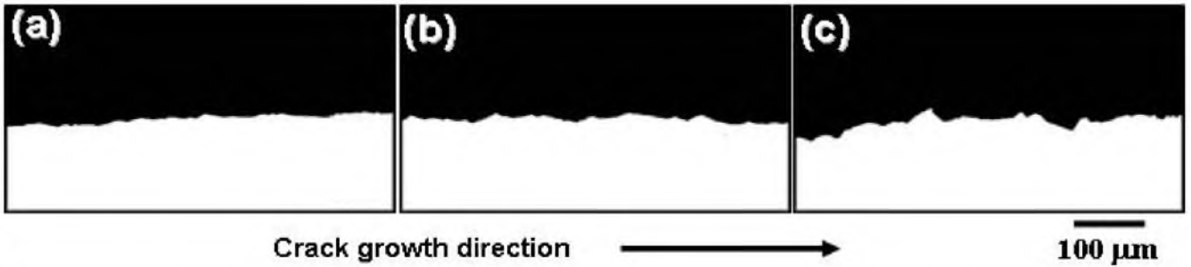
Fig. 3 Fatigue crack surface profile in UFG Al-6%Mg-0.3%Sc alloy developed at various distances, \Delta L , from the initial crack tip: (a) \Delta L = 4 mm ( \Delta K \sim 7 MPa m^{0.5} ); (b) \Delta L = 7 mm ( \Delta K \sim 9 MPa m^{0.5} ); (c) \Delta L = 13 mm ( \Delta K \sim 18 MPa m^{0.5} ).
