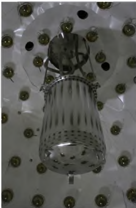
Figure 2. The Liquid Scintillator Veto (LSV). The picture shows the cryostat of the DarkSide-50 LAr TPC hanging from the top.
